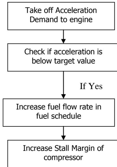
**Figure 8:** Flow chart for increasing fuel flow rate by the life enhancing system [16]
