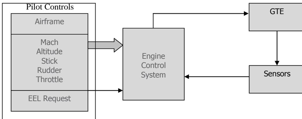
**Figure 9:** Control schematic for extending life [15]
