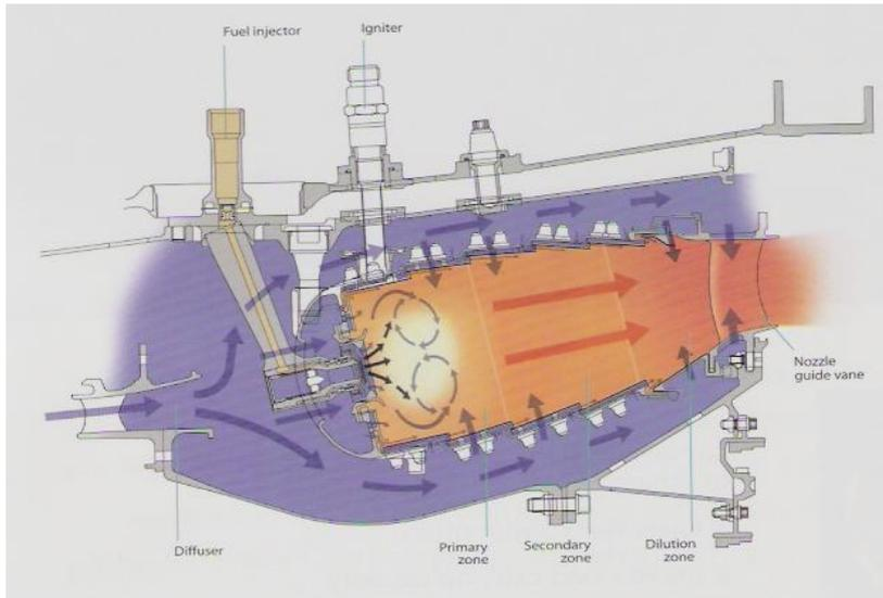
**Figure 7:** Combustor Chamber [14]
