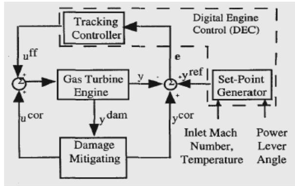
**Figure 4:** Control schematic using critical models [4]
